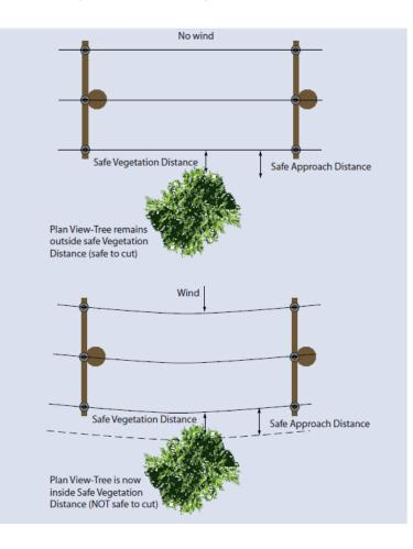
Figure 3 – Conductor Sag and Sway (Section Elevation)
