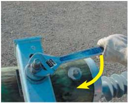
Adjust the spanner whilst placed on the nut/bolt to remove slack in the jaws.
