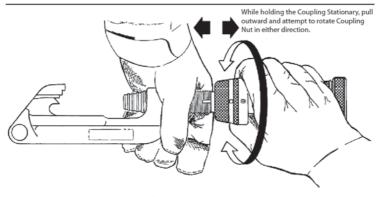
If coupling nut turns more than 4' (about 3.2mm [1/8in]), the "Fail Safe" is broken. DANGER DO NOT FIRE THE TOOL.
