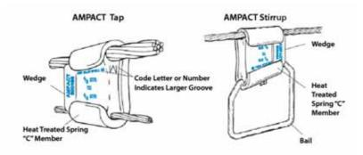
When connecting two different size conductors the wedge will have a letter or number that indicates the larger groove (see picture above)
