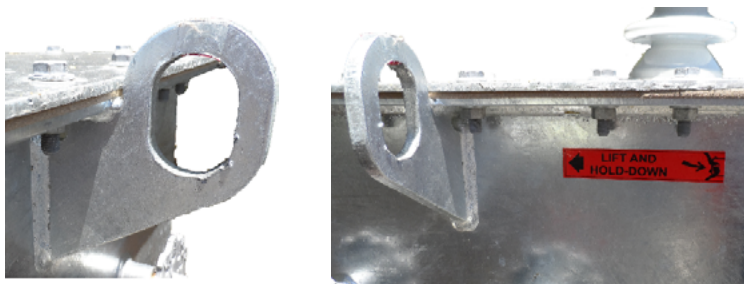
Lifting points on 22kV transformer
