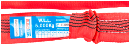
Round sling with the cover pulled back to inspect tag details
